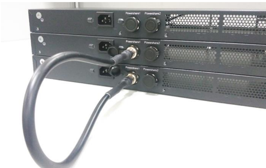
Figure 3-11 Connecting Cables Among Three Switches 2
