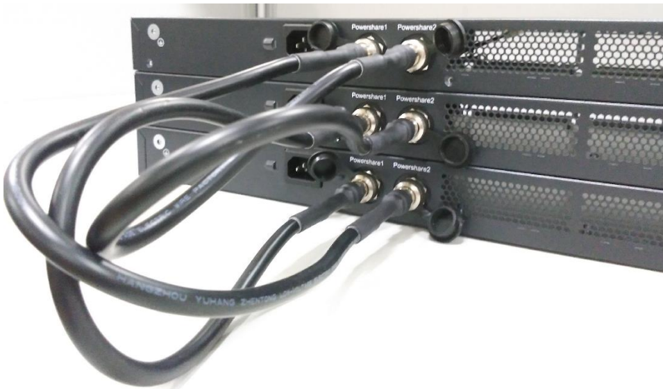
Figure 3-12 Connecting Cables Among Three Switches 3
